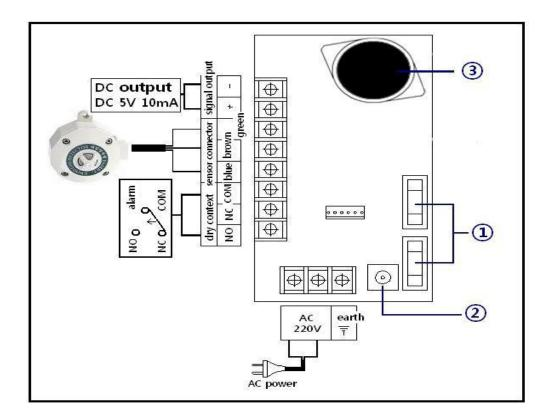
① AC FUSE (2EA): 220V 1A glass tube (When it has blown, RED warning light of the fuse gets lit)
